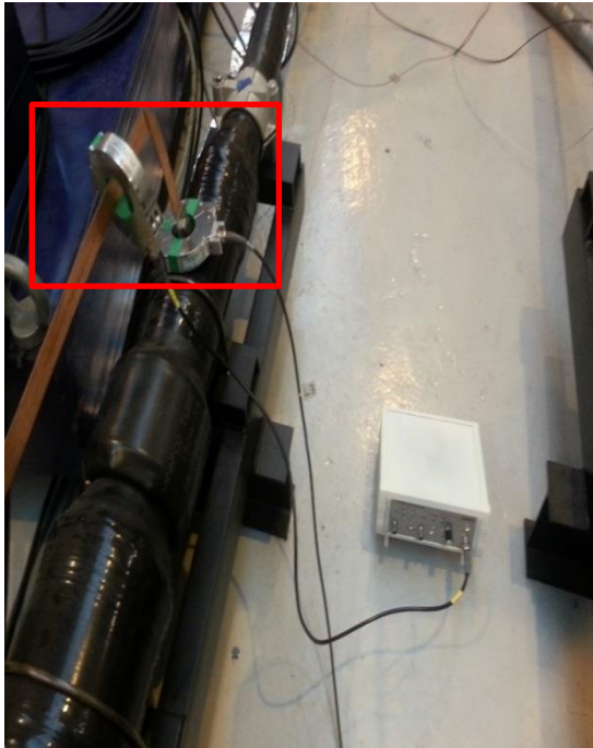
Positioning of three types of OLPD Sensor on the cable test Rig
